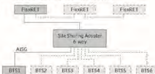
Configuration example with Site Sharing Adapter 86010155
