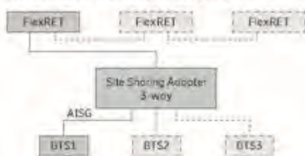
Configuration example with Site Sharing Adapter 86010154
