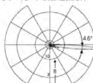
Vertical Pattern 0°–10° electrical downtilt
