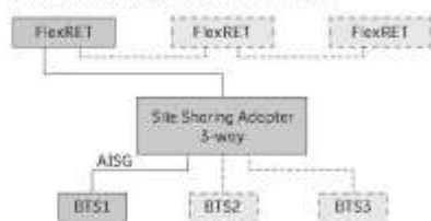
Configuration example with Site Sharing Adapter 86010154
