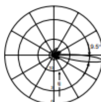
Vertical Pattern 6° electrical downtilt
